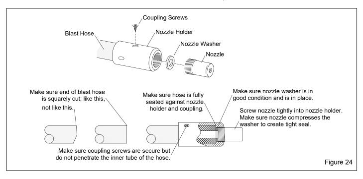
**7.2.3** Replace the nozzle when its orifice (the smallest inside diameter) has increased by 1/16" or sooner if blast pressure noticeably diminishes. Make sure the nozzle washer is in good condition and in place before screwing the nozzle into the nozzle holder. Make sure the nozzle is screwed tightly into the nozzle holder; if nozzle is not tight against the nozzle washer, thread erosion will occur and nozzle will fuse to nozzle holder.
