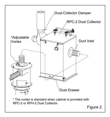
**1.7.3 RPH-2 Dust Collector:** The RPH-2 is available in 600 cfm and 900 cfm models. It is set up and operate the same as the RPC-2, as shown in Figure 2, but instead of a dust drawer, the collector sits atop a hopper, which provides additional dust storage, and empties into a drum. Refer to manual number 21449.
