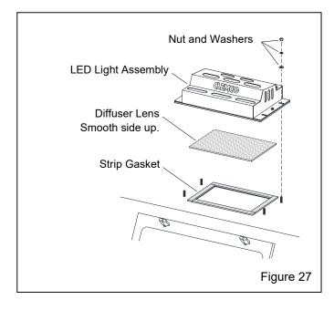
**7.7.2.3** Set the light assembly on the diffuser and reattach it using the existing nuts and washers.
