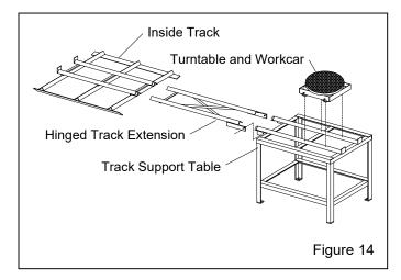
**3.5.2** Place the inside track in the cabinet over the existing grate, as shown in Figure 15. The workcar stops must be on the opposite side from the entry door.
