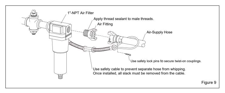
**2.9.3** Refer to the dust-collector operations manual and connect a compressed-air line to the pulse manifold.
