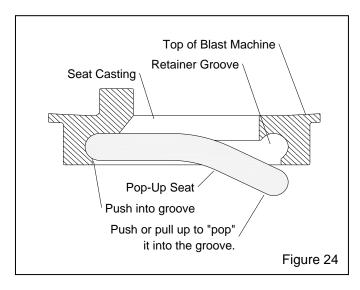
**6.8.2** Push the new seal all the way through the port and then fit it into the retaining groove. For the last few inches, pull up on the seal and allow it to pop into position.
