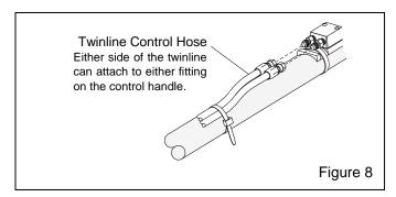
NOTE: When attaching Clemco <u>twinline</u> hose to any Clemco valves either side of the twinline hose can be attached to either twinline fitting on the valve.
