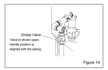
**3.5.2** Closing the choke valve while blasting lowers pressure in the pusher line from the pressure in the vessel. Closing the valve forces abrasive through the metering valve to clear minor blockage, such as damp abrasive, or is used to rapidly empty the machine at the end of the day.
