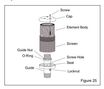
**6.9.5** Make sure the guide nut is fastened tightly to the guide.
