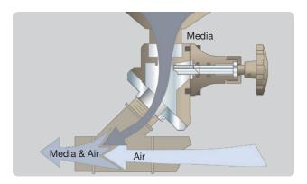
The Manual Quantum Valve (MQV) handles all types of media: mineral, slag, and metallic. Its design allows for precise metering and easy maintenance. It fits machines with 3-cuft to 20-cuft pressure vessels.
