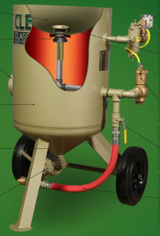
Self-cleaning exhaust muffler greatly reduces bleed-off noise.
