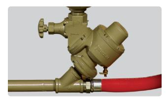
The Auto Quantum Valve (AQV) is for pressurehold remotes and pressure-release remotes equipped with an abrasive cutoff system. Abrasive cutoff permits shutting off abrasive to blow down surfaces with air. Available in pneumatic or electric.
