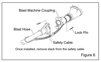
**2.6.1** Connect the blast hose from the cabinet hopper to the coupling at the bottom of the blast machine. Make
