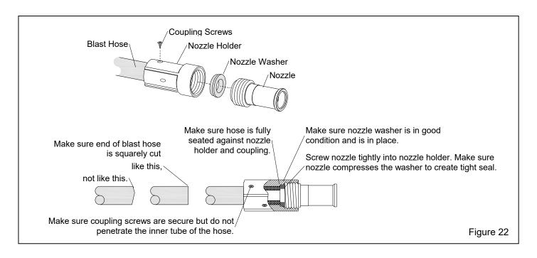
**7.2.3** Replace the nozzle when its orifice (the smallest inside diameter) has increased by 1/16", or sooner if blast pressure noticeably diminishes. Make sure the nozzle washer is in good condition and in place before screwing the nozzle into the nozzle holder. Make sure the nozzle is screwed tightly into the nozzle holder; if nozzle is not tight against the nozzle washer, thread erosion will occur and nozzle will fuse to nozzle holder.
