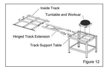
**3.4.2** Place the inside track in the cabinet over the existing grate, as shown in Figure 13.
