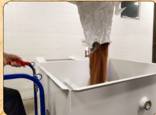
4) Abrasive is released into hopper.
