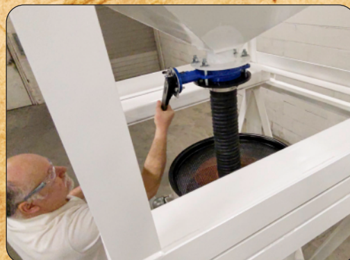
6) Butterfly valve is opened, loading abrasive into vessel.
